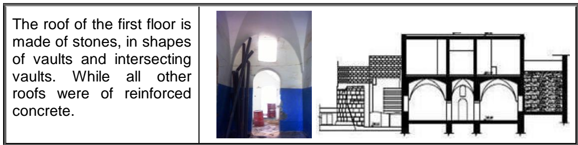
Fig. 6. The materials used for constructing the building in its beginning
