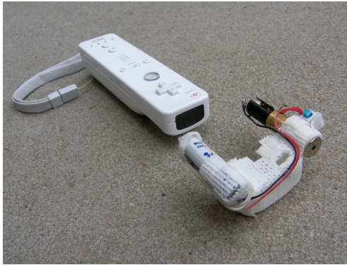
Figure 5 Wiimote® and the laser pointer attachment
